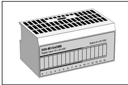
Each signal is isolated from the logic circuits by an optocoupler and filtered with a low-pass filter. The inputs have a programmable filter time.
