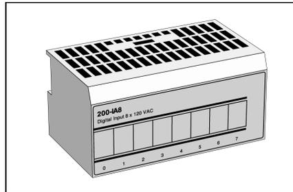
The input signals are sampled at intervals determined by the filter time. The signal status is changed only if two consecutive samples are the same. The filter time is set with the programming software.
