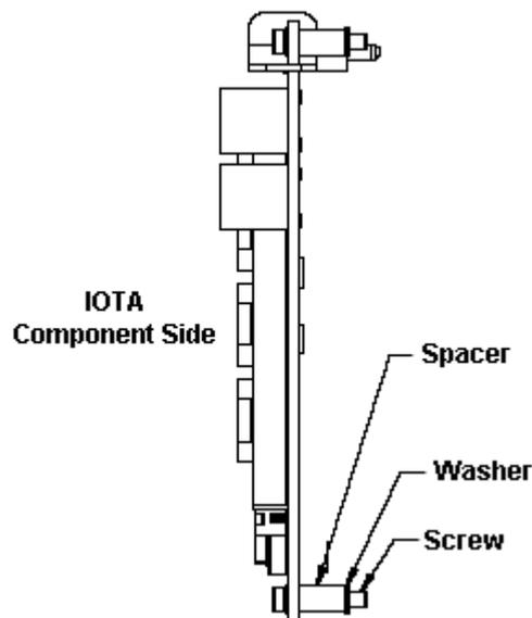
3. Tighten the screws in terminals **24 Vdc +** and **COM** (logic ground) to the vertical bus bar to connect the cabinet resident 24 Vdc power supply to the IOTA.
