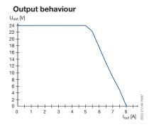
Output curve at  $T_a = 25 \text{ °C}$
