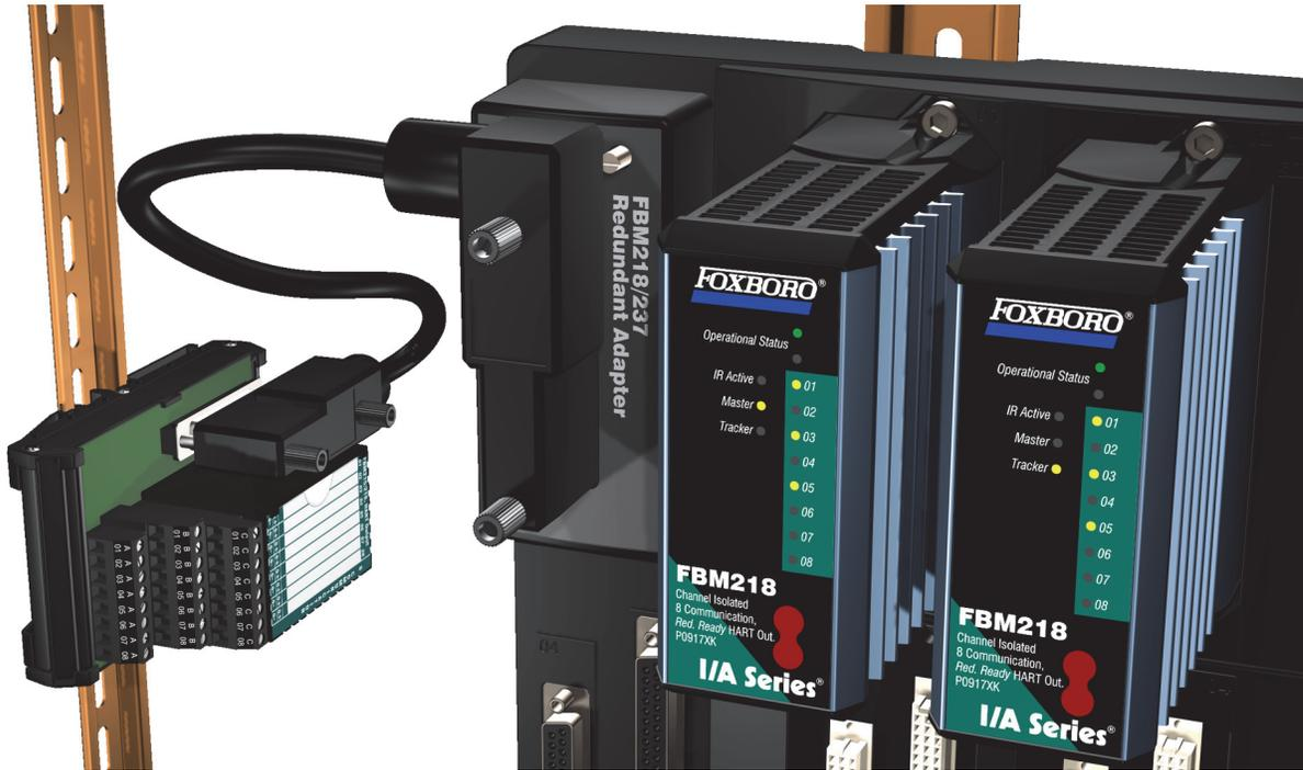
The FBM218 offers redundant modules for eight output channels, each providing a 4 to 20mA output signal or a digital HART® signal superimposed on a 4 to 20 mA analog output signal.
