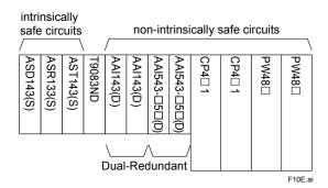
The total sum of the factors for this installation plan is less than 65 as shown below, hence, the acceptance of this plan is ensured:
