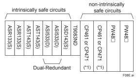
\*1: A dual-redundant configuration is enabled by using 2 identical modules with same model code (CP461 or CP471).
