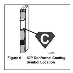
**Note:** Boards installed and maintained in a G1 (mild) control room environment (defined by the ISA Environmental Severity Classification) do not need this added protection.
